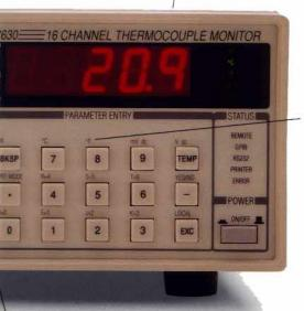
Each channel may be independently configured for thermocouple type, display units, and nominal temperature. The first four channels can drive rear panel analog outputs with variable offset and gain.
